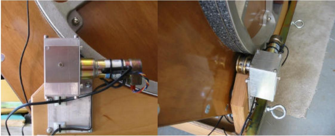
Figure 6 Alt motor assembly
